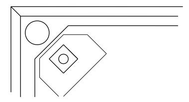
8- Remember that you now need a full surface top plate for the turntable to sit on. The motor is no longer supported by the base and must stand on its own. If you have raised the base of the turntable up by more than the standard 17 mm leg you must raise the SAMA by the appropriate amount to maintain the same relationship of motor to chassis
