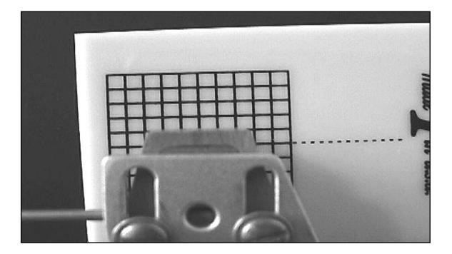
FIG #2: THE PROPER WAY TO ALIGN A CARTRIDGE, ALIGN THE CARTRIDGE, NOT THE TONEARM HEADSHELL!
