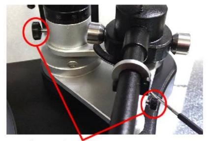
Loosen these two screws to adjust VTA and tighten when set
