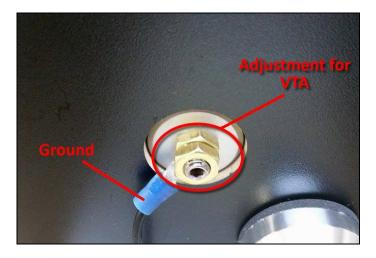
Loosen the nut, remove the ground wire, then you may adjust the height by turning the brass nut.
