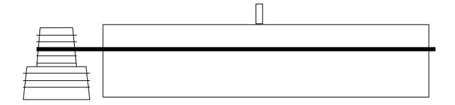
• Level the turntable using a 9" or 12" long bubble line level placed next to the spindle on the platter. The feet rotate in their sockets and will move
