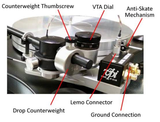
Tracking force is adjusted by moving the tonearm counterweight forward and back on its shaft. If your cartridge is overly heavy and the counterweight is all the way back, you can order a heavier weight from your dealer. Half way back is fine as is the middle third of the stub.
