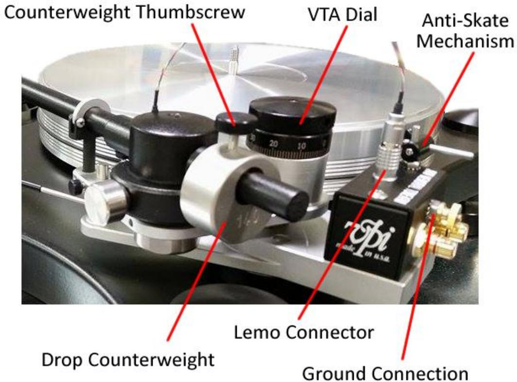
Tracking force is adjusted by moving the tonearm counterweight forward and back on its shaft. If your cartridge is overly heavy and the counterweight is all the way back, you can order a heavier weight from your dealer. Half way back is fine as is the middle third of the stub.
