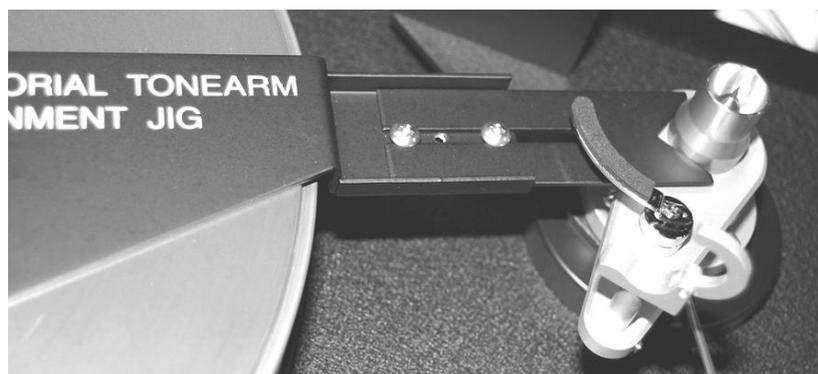
**MAKE SURE THE MALE POINT IS IN THE CENTER OF THE FEMALE CUP, IT SHOULD FEEL SOLID BUT YOU SHOULD BE ABLE TO SLIDE IT SIDWAYS AND THE ARM RAISES AS YOU GO FROM THE CENTER TO THE SIDES OF THE FEMALE BEARING. IT IS AN INVERTED CONE.**
